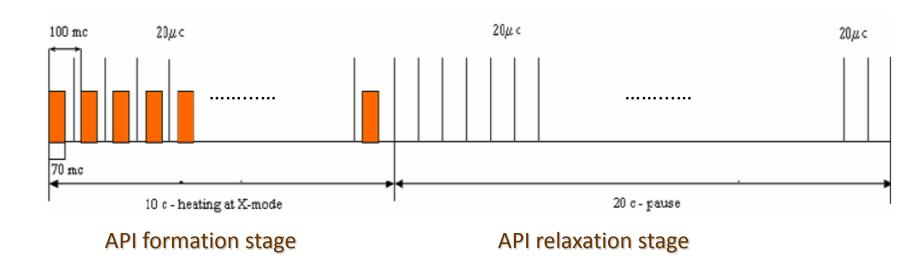
The HAARP facility operated with period 15(30) s. This period consisted of (i) 70 ms pulses separated by 30-ms pauses and short (20  $\mu$ s) sounding pulsed during first 3 (10) s, and (ii) 20  $\mu$ s sounding pulses with IPP 20 ms during the following 12 (20) s. The pulse train (i) used for study of the API development and stationary states, while the train (ii) used for the relaxation stage. The X-polarization of the heating and sounding modes was applied.
