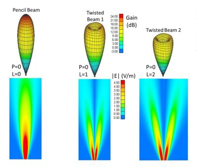
Figure 5. HF array beam twisted-beam modes formed by exciting the HAARP array with the phase equal to integer multiples of the azimuth angle from the central point of the array.
