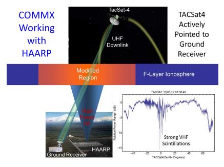
Figure 9. Satellite transmissions from TACSat4 along a propagation path in the ionosphere illuminated by the high power HAARP beam. The strong 253 MHz occur with the satellite orbit carries the COMMX/TACSat4 transmissions through the region of artificial ionization by HAARP.
