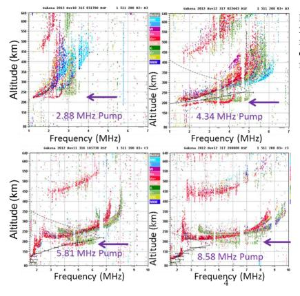
Figure 4. Tuning HAARP to the 2nd, 3rd, 4th, 6th gyro harmonics to form plasma clouds near multiples of 1.44 MHz electron cyclotron frequency.
