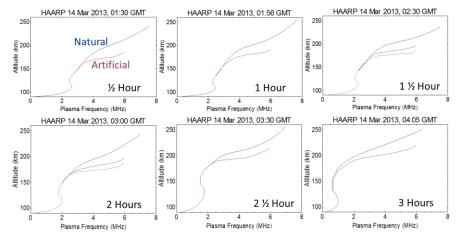
Figure 8. Natural and artificial ionization profiles of the ionosphere provided the HAARP ionosonde. The altitude of the plasma cloud remains offset from the background layer by about 40 km for the period of power extended high HF pumping at 5.8 MHz.
