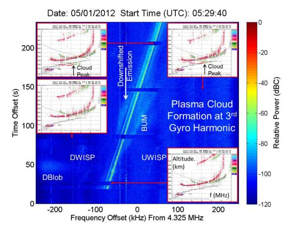
Figure 3. Stimulated electromagnetic emissions (SEE) observed during a  $3^{rd}$   $f_{ce}$  frequency sweep that produced artificial plasma clouds.
