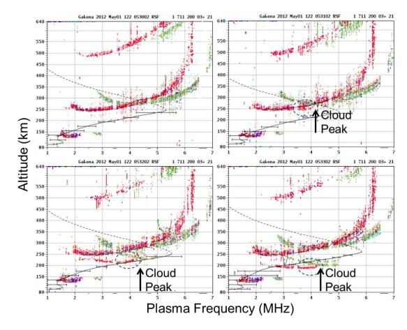
Figure 2. Artificial ionization cloud formed with peak plasma frequency at the 3<sup>rd</sup> electron gyro harmonic around 4.325 MHz. The altitude of the cloud descends with time.
