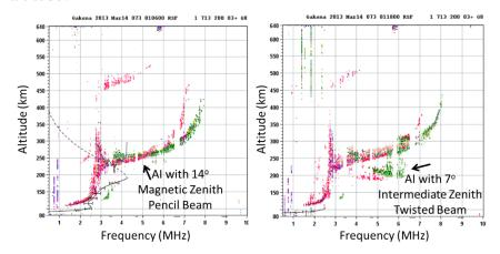
Figure 7. Ionosonde signatures of artificial ionization (AI) with a 5.8 MHz pencil beam points at the magnetic zenith (MZ) and a 5.8 MHz twisted beam pointed between MZ and vertical. The transmissions started at 01:06 GMT with the pencil beam and 01:10 GMT with the twisted beam in virtually the same background ionosphere.
