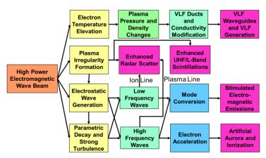
Figure 1. Four basic processes that describe the physics of high power interactions with the plasma in the ionosphere. The thresholds for each process increases from top to bottom. Enhancement of self-action effects involve feedback and coupling between two or more processes.
