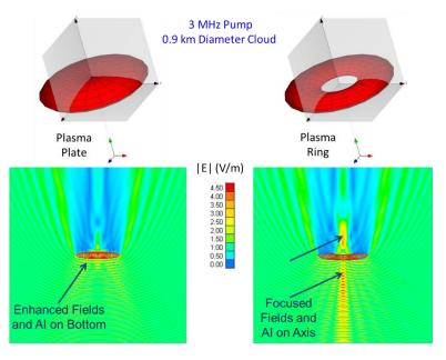
Figure 6. Numerical electromagnetic simulations of plate and ring distributions illuminated by a 3 MHz electromagnetic wave. The plasma plate intensifies the incident electric field on the bottom. The ring structure produces plasma breakdown above and below the cloud height.
