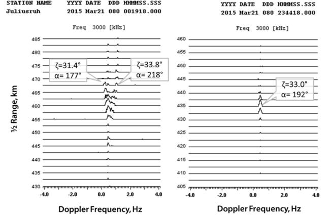
During quiet conditions on the path between Pruhonice and Juliusruh (the right panel), the HF pulse arrives at an apparent range of 2x435 km, zenith of  $33^{\circ}$  and azimuth  $192^{\circ}$ .
