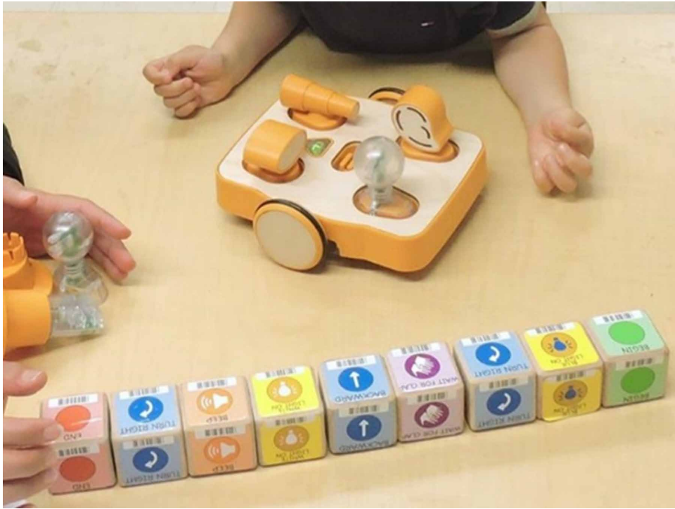
Figure 1. Example KIBO robot and interlocking wooden programming blocks
