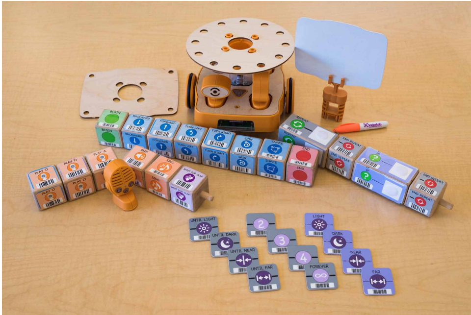
Figure 2. KIBO robot with programming blocks and accessories
