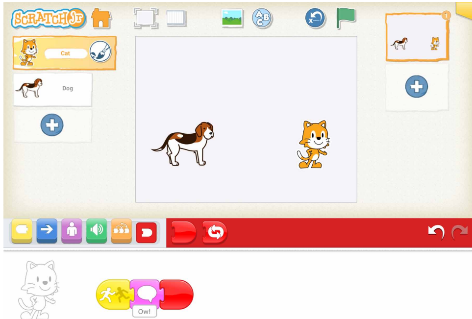
Figure 4. A ScratchJr program showcasing the “Start on Bump” block
