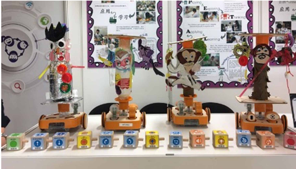
Figure 2. A KIBO robotics project programmed with wooden blocks
