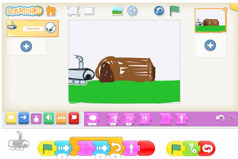
Figure 1. The ScratchJr interface with Henry's train. In this photo, the train is programmed with a repeat loop to disappear 5 times while it goes in the tunnel and then appear at the end.
