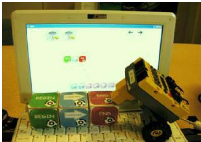
Figure 3. Tangible and on-screen elements of the CHERP language developed at Tufts University.
