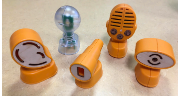
Input/output modules (distance, sound, and light sensors, lightbulb, sound recorder)
