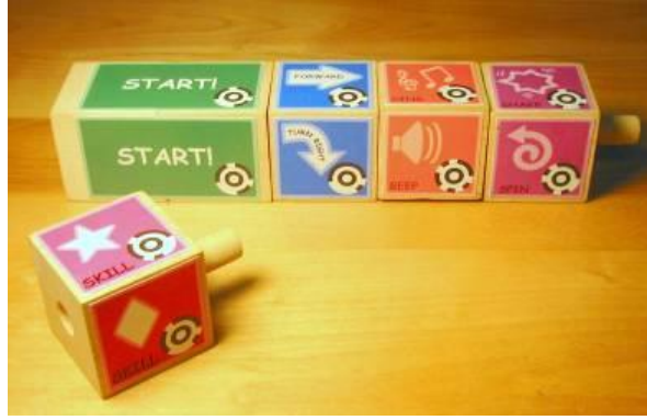
Figure 3.7: To address drawbacks of the wooden train track blocks for use in kindergarten, I redesigned the language to use interlocking wooden cubes with pegs on one side and holes on the other. Mary Murray, an intern at the Boston Museum of Science and a masters student at the Massachusetts College of Art and Design was the originator of this concept.
