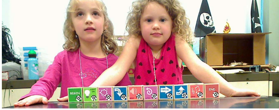
Figure 1.1: Tern is a tangible programming language that allows children to construct physical algorithmic structures using interlocking wooden blocks.
