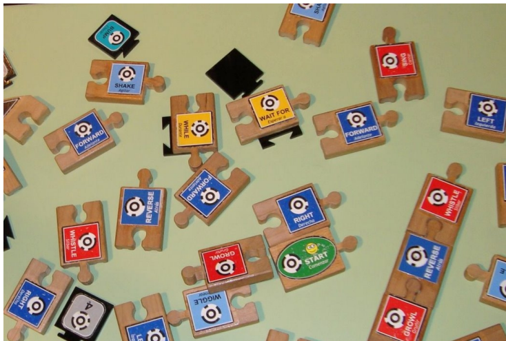
Figure 2.7: Our tangible programming interface, Tern, consists of a collection of wooden blocks shaped like jigsaw puzzle pieces.
