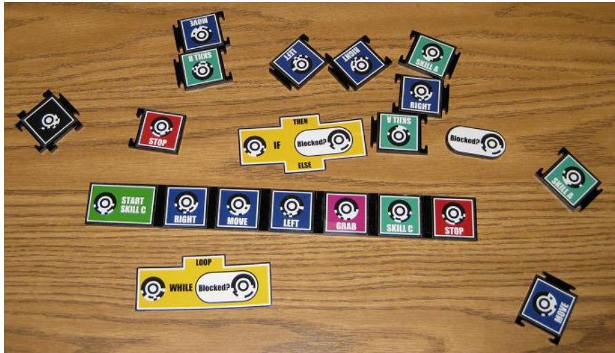
Figure 3.4: I built the earliest Tern prototypes using laser cut plastic and a jigsaw puzzle piece metaphor. The language itself was modeled after the educational programming language, Karel the Robot. This picture shows a recursive subroutine.
