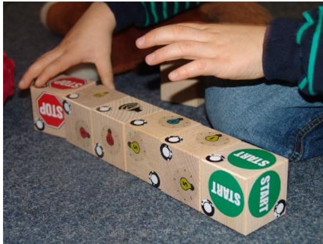
Figure 2.5: An early prototype of the Tangicons (Scharf et al., 2008) system from the University of Lubeck which uses my TopCode library to create a game for kindergarten children that combines physical exercise with simple programming activities.
