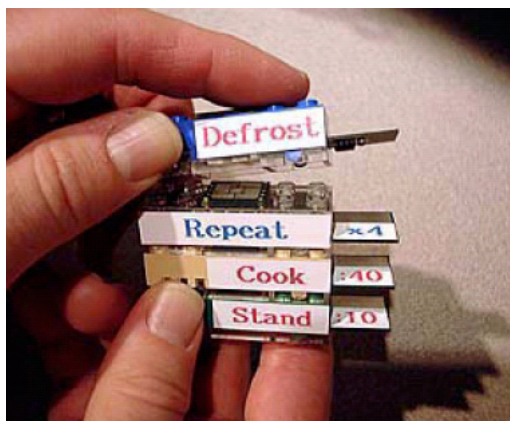
Figure 2.4: Tim McNerney’s Tangible Computation Bricks (McNerney, 2000) features a LEGO-like construction kits with embedded microprocessors that allow children to experiment with programming concepts in real-time.
