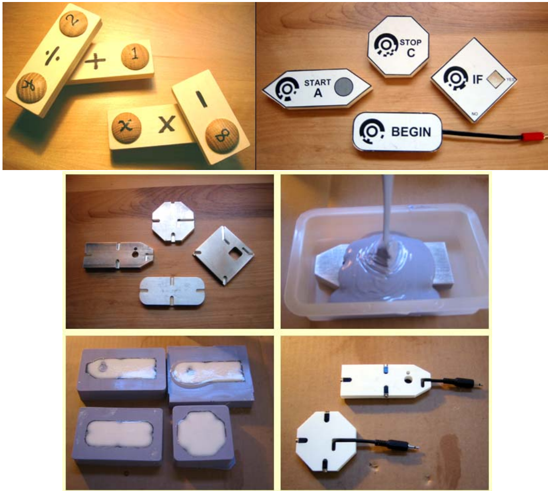
Figure 3.1: Early prototypes constructed of wood (top left) and foam core (top right). The bottom four pictures illustrate the process of creating molded urethane parts from machined aluminum originals.
