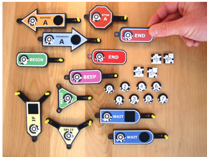
Figure 3.2: The final Quetzal prototype consisted of flat tiles laser cut from an acrylic sheet. Printed paper faceplates show both a human-readable statement name and a computer vision fiducial. The statements can be chained together at pivot points at the end of rigid connection arms.
