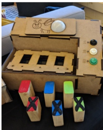
Fig. 1. CRISPEE platform (center) and gene coding blocks (front) are used to simulate changing the light color emitting from a bioluminescent animal.
