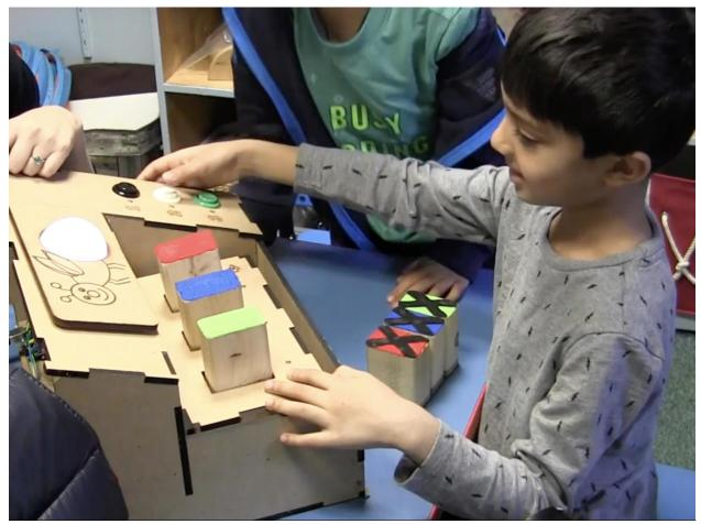
Figure 4. Yanni (foreground) tests a CRISPEE program Green On, Blue On, and Red On blocks, creating a firefly with a glowing White light. The Off (or X) blocks are arranged on the table in front of him.
