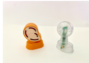
Input/output modules (sound sensor and lightbulb)
