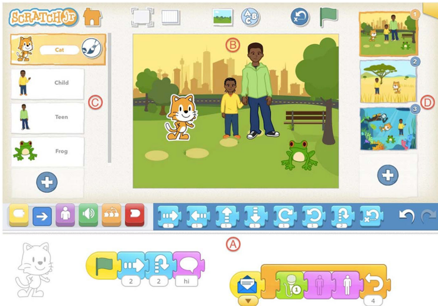
Fig. 2 A screenshot of the ScratchJr interface. The interface consists of a a programming “editor,” or workspace, b a stage where characters execute programs, c a list of all the characters on the stage, and d a gallery of up to four pages, each with a new stage, workspace, and character list to continue the project
