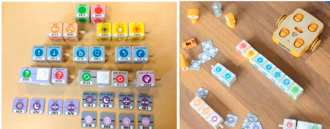
Fig. 3. Blocks for programming KIBO and a sample KIBO program (sequence of spin, shake, move backward, move forward, and turn on a red light). (For interpretation of the references to color in this figure legend, the reader is referred to the Web version of this article.)
