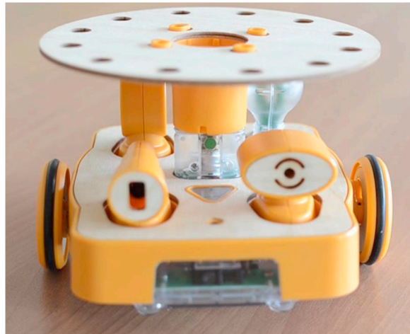
Fig. 2. KIBO robot with sensors, light output, and turntable platform attached.
