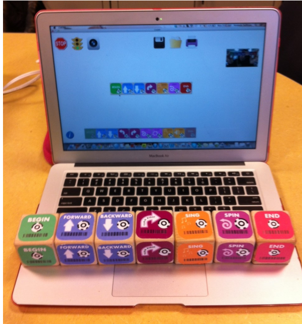
Figure 5.2: Sample program created with CHERP blocks and shown on computer interface
