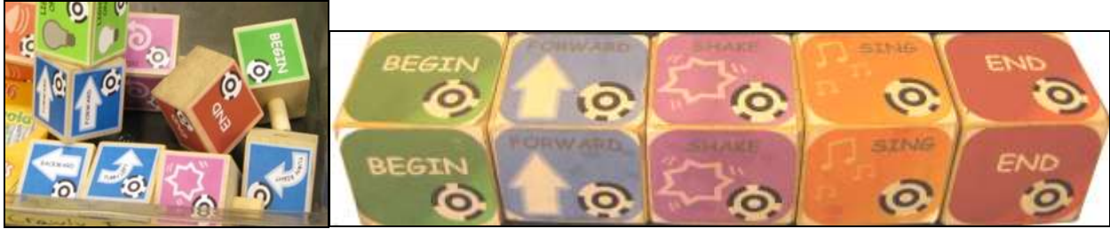
Figure D2. CHERP's tangible interface. It consists of interconnecting wooden blocks.
