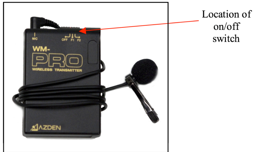
Figure 3.5: The Azden wireless lapel microphones (WL/T-PRO) used in this project. The on/off switch at the top was taped down with masking tape to prevent it from accidentally getting switched off while the students were wearing it.
