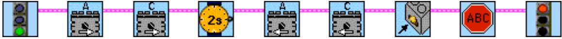
Figure 1.3: Sample ROBOLAB program. This program tells a car (built around the RCX) to go forward for two seconds then to go backwards until the touch sensor is pushed, and then stop.
