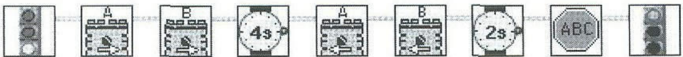
Figure 2. A simple program in ROBOLAB. This program would tell a car built with two motors to go forward for 4 seconds, then to go backwards for 2 seconds, then to stop.
