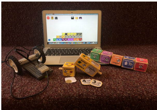
Fig. 2 CHERP interfaces and LEGO WeDo robotic kit. Computer screen shows graphical CHERP interface, and blocks represent tangible interface
