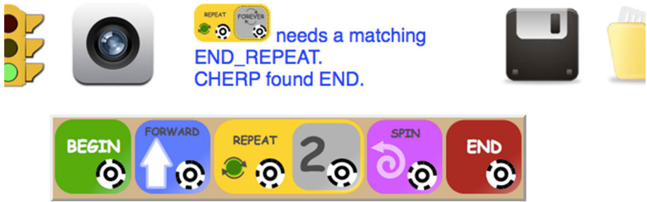
Fig. 15 CHERP graphical interface warning. This computer warning occurs when a repeat loop is syntactically incorrect and will not compile. The message prompts the user to include the correct block
