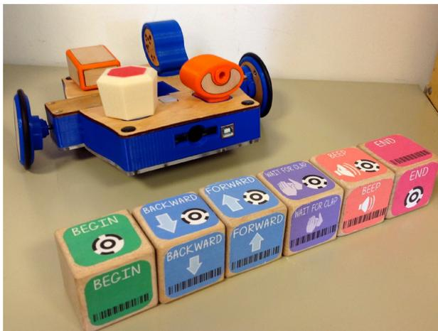
**Figure 1 KIWI Robot and CHERP Programming Blocks**
