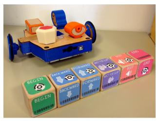
Figure 1 KIWI Robot and CHERP Programming Blocks
