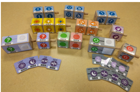
Figure 2. KIBO’s tangible programming language. Each block has a unique barcode that is scanned by the robot.
