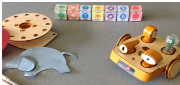
Figure 1. KIBO robot with a sample block program, art platforms, and art supplies for decorating.
