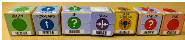
Figure 3. This figure provides an example of a conditional statement with KIBO.
