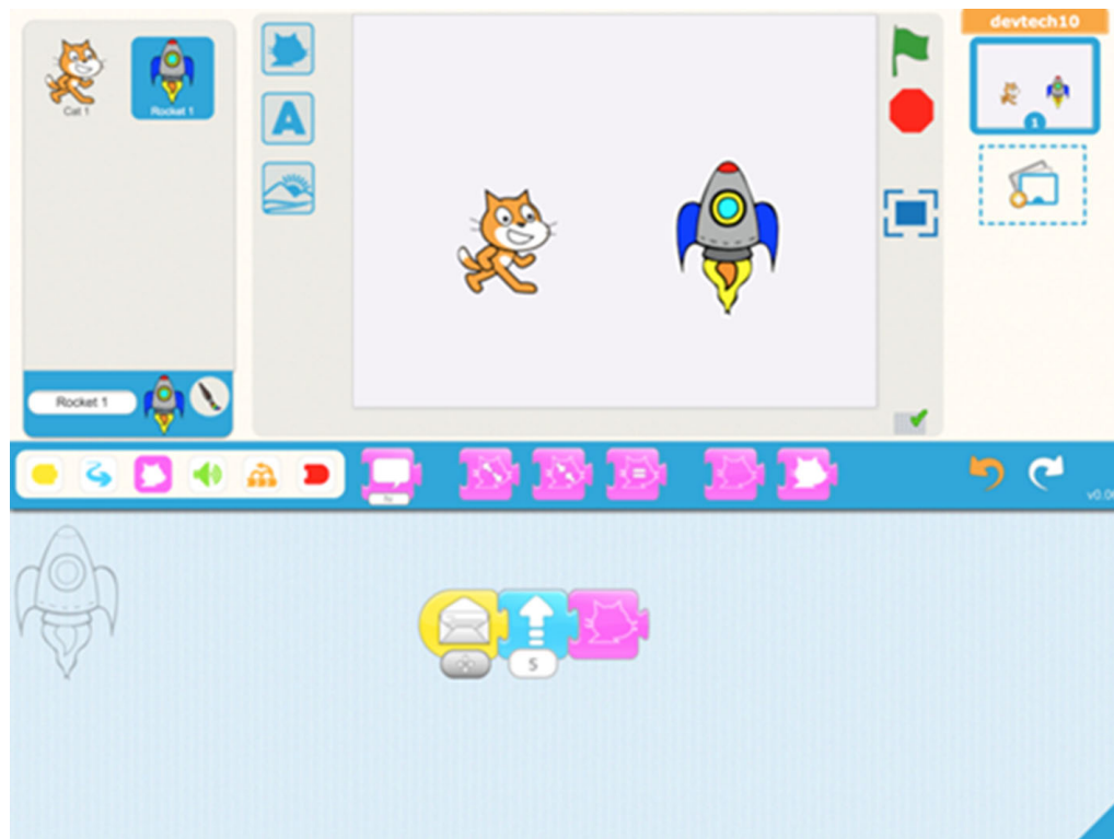
Fig. 4 Same ScratchJr project as in Fig. 1 but this time showing the Rocket 1 script that “receives the message” from Cat 1 and then makes it move up five spaces and hide. (Color figure online)
