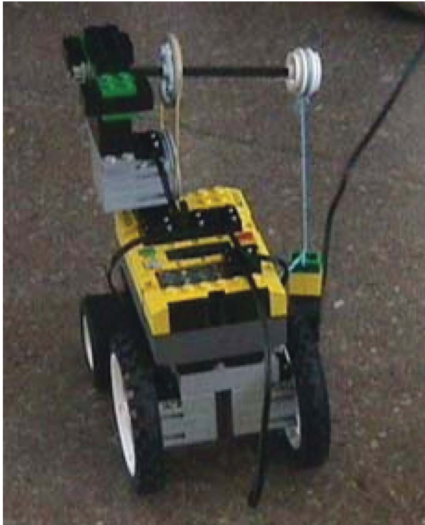
FIGURE 4 The RCX programmable brick with wheels, motors, and sensors (color figure available online).
