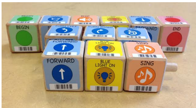
Figure 2. Each KIBO programming block has a different barcode. The robot’s embedded scanner reads each barcode and sends the instructions to the robot.
