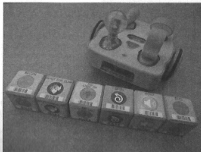
Fig. 10.1 The KIBO robot with sensors, light output, and sample block program
