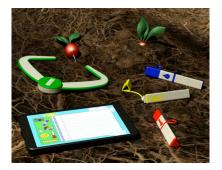
Figure 1, the digital lab notebook and a collection of scientific probes for measuring size, humidity, pH, and temperature.
