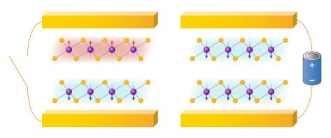
**Fig. 1** | Schematic of electrically induced antiferromagnetic-to-ferromagnetic state switching in atomically thin Crl<sub>3</sub>.
