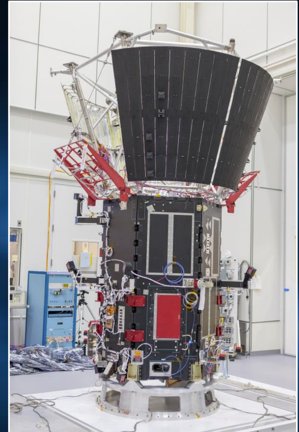
Solar Array Cooling System Integration – Spacecraft Closed for Alignment Measurements
