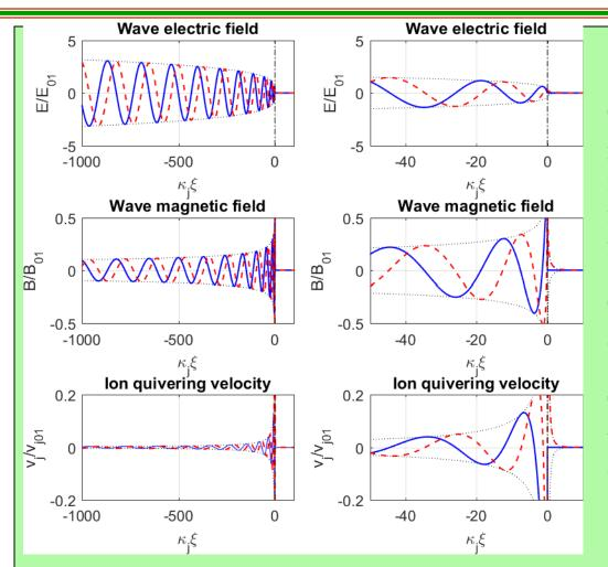
The real parts (blue solid lines) and imaginary parts (red dashed lines) near the resonance layer at  $\xi = 0$ for a linearly decreasing magnetic field.
