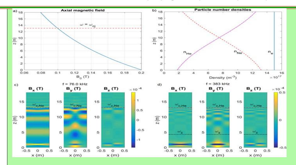
Propagation of EMIC waves in two ion Ne-He plasma using plasma parameters relevant for the LAPD device.
