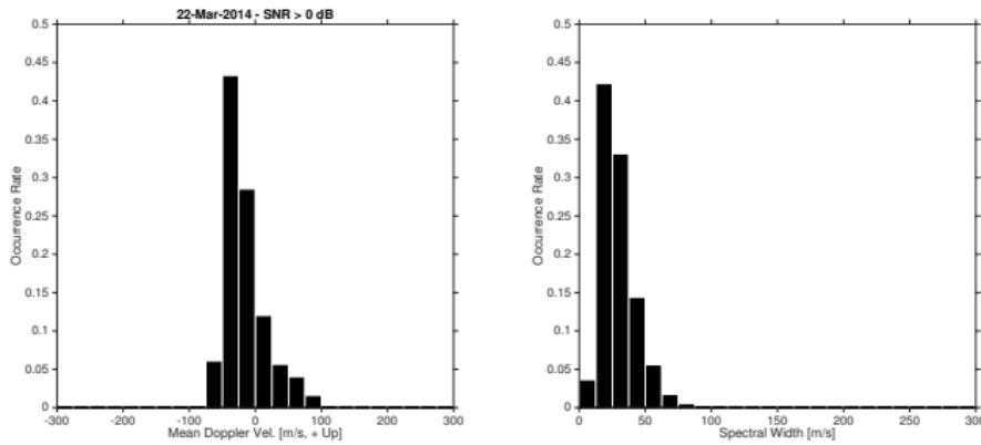
Histograms of mean Doppler velocities (+ upward) and spectral widths estimated from the observations made by MELISSA on March 22, 2014.
