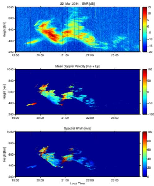
Examples of parameters derived using the MELISSA radar on March 22, 2014. SNR (top panel), vertical velocity (middle panel) and spectral width (bottom) panel.
