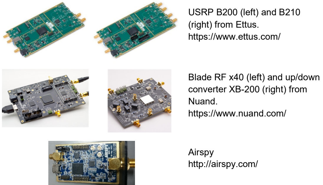
Figure 2: Software-defined radio device which we now test for new beacon receiver.
