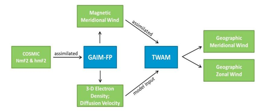
TWAM is based on a first-principles data assimilation model for the thermospheric wind.
