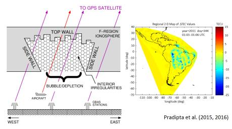
Steep TEC gradients can come from the side walls as well as irregularities inside the bubble (may cause scintillation and/or loss-of-lock).
