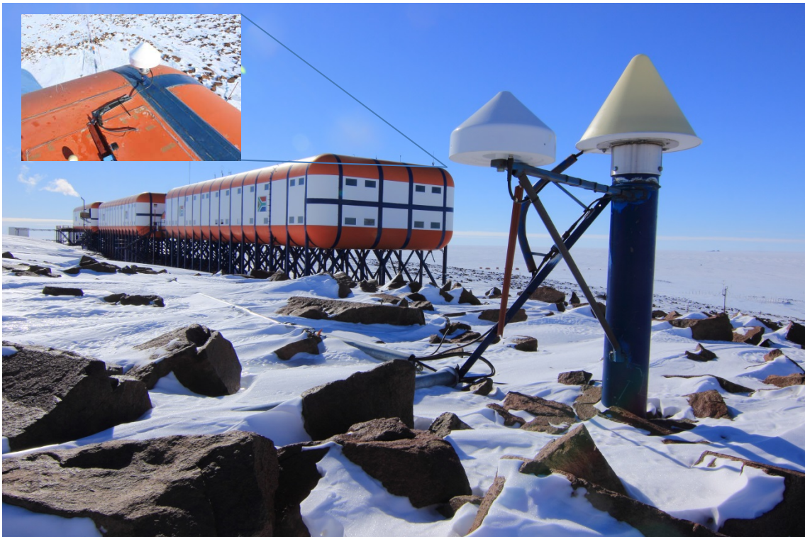
Figure 1. Co-located GNSS receivers at SANAE, the South African Polar Research base in Antarctica. In the foreground is the antennas of the GPS and Novatel Scintillation receivers, and on the roof of the base (insert) is the antenna shared by the Septentrio PolaRxS PRO GNSS receiver and the software-based GNSS data acquisition system.
