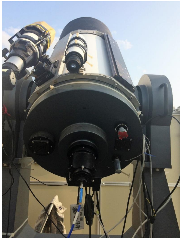
Ocean Optics QE65000 spectrometer connected to primary optic of AFIT telescope via optical fiber
